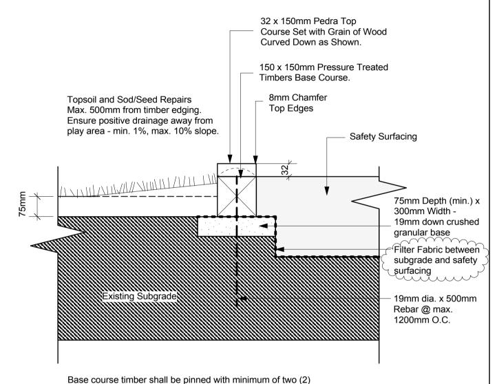
19mm dia. rebar @ max. 1200mm O.C.
